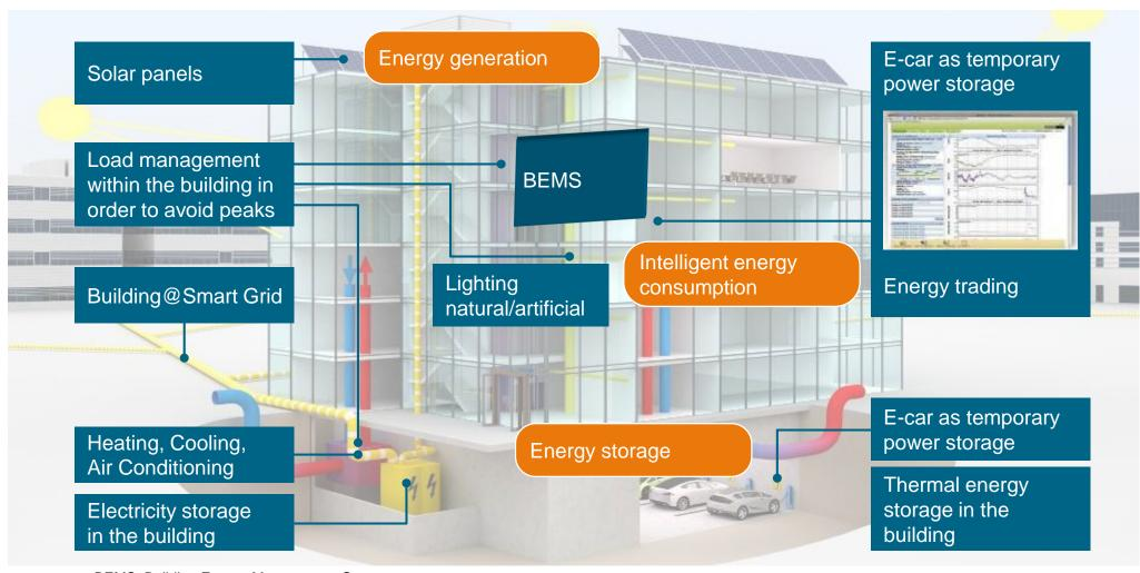
Source: BT BAU BEMS: Building Energy Management System
